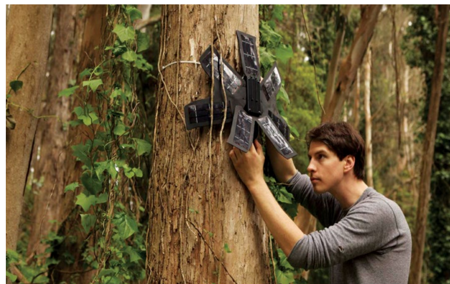
Forest sensors. New technologies like forest sensors can measure the health of the forests, wildlife and bird populations while listening for chainsaws and gunshots.
